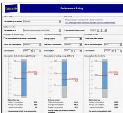
Performance rating tool for comparing the energy and water consumption of specific buildings to the national average of buildings of the same type.
